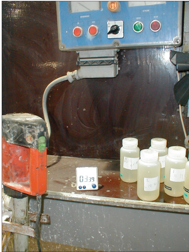
Figure 6.2 Sample solutions. The solutions in the baths (samples in plastic bottles) are analysed. This makes it possible to add the correct amount of chemicals to have the baths operate properly. (Photo: Roskilde Municipality Environmental Inspection office)
