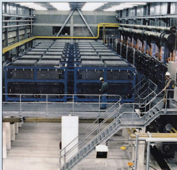
Figure 7.1 Chlor alkali industry. View of a membrane cell room equipped with bipolar electrolysers [source: the BREF document].
