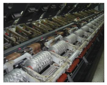
Figure 1.4 The spinning machines.
