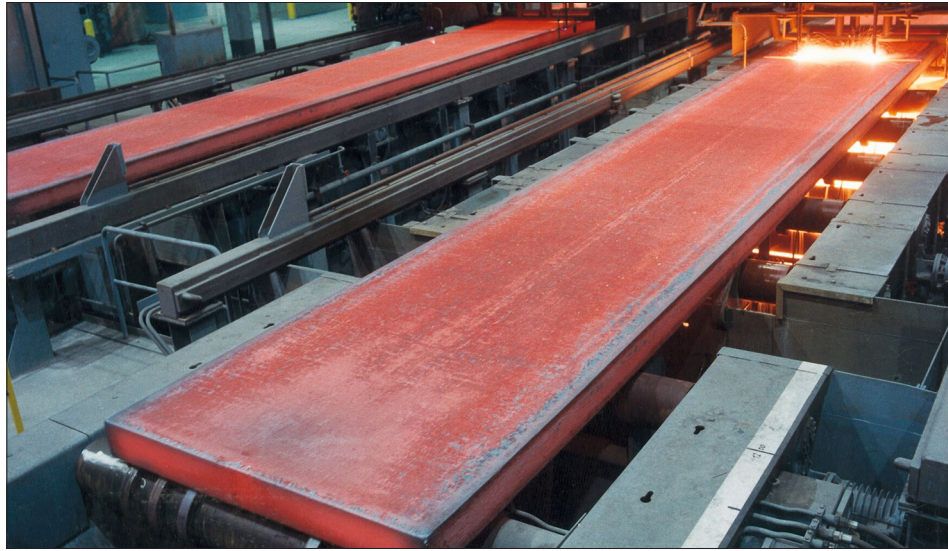
Figure 2.2 Steel heavy plates. Technical solutions used in the rolling mill enable manufacturing of many categories of steel plates with various properties and applications. Photo: Stahl-Zentrum.
