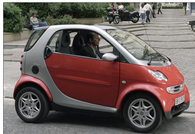
Figure 4.4 The Smart car (Example 4). This car for city traffic is small (2.5 m) easy to park and uses little fuel (about 4 litres/100 km). It contributes to a reduced resource flow.
