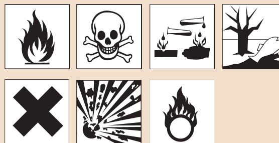
Figure 3.4 Labels for chemical management. The labels are used to communicate the risks connected with the chemicals. The labels from top left indicate flammable, poisonous, corrosive, ecotoxic, allergic, explosive and oxidising. For each category there are strict rules for classification e.g. in terms of LD_{50} on rats, or flame point, etc. The Chemicals Inspectorate in each country maintains databases where the regulations for storing, handling, and disposing of each chemical can be found.
