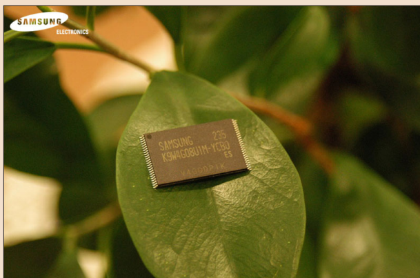
Figure 10.3 Lead-free semiconductor from Samsung. 4Gb NAND Flash memory to be used in products such as mobile phones, digital still cameras, handsets, MP3 players and USB Flash drives, etc. Photo: © Samsung.
