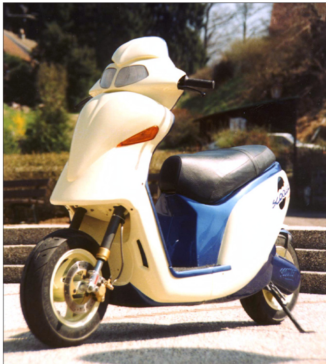
Figure 4.7 Electric scooter (Example 8). This scooter (the Scooter) runs on battery for 95 km on 45 km/h. Costs is about 10% of running a traditional gasoline motor scooter.
